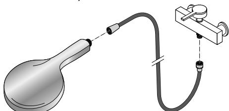
2. Screw the end of the hose with the knurled nut to the fitting and the end with the elongated screw piece to the shower head.
